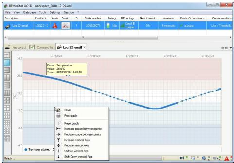
By passing the mouse cursor on the point representing the measure, the exact value of the measurement is displayed and the date and time of the measurement.
