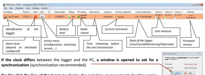
Double-click the line of the logger to display the real-time measurements for this Logger.
