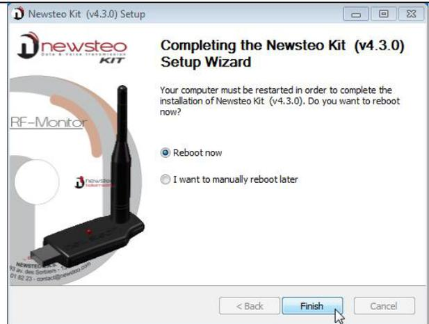
In the first window select a language then, for a quick installation, **keep the default settings by validating the successive windows from setup program.** By the end of installation, **keep the option "Reboot now" and click "Finish".**
