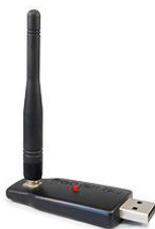
4. The GAT, the loggers and the RF-USB key must be on the same radio channel (the GAT and the USB key are factory set on radio channel 1 when delivered)
