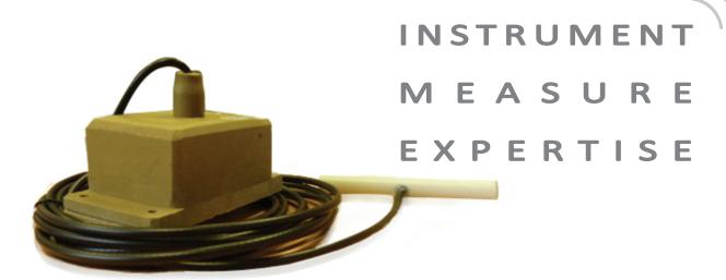
The concrete quality depends on the respect of the setting and curing. Newsteo has developed the Newsteo Builder, in partnership with Lafarge, the Newsteo Builder, which allows measuring and recording of the temperatures and the shrinkage, at the first hours of the setting and during the following years.
