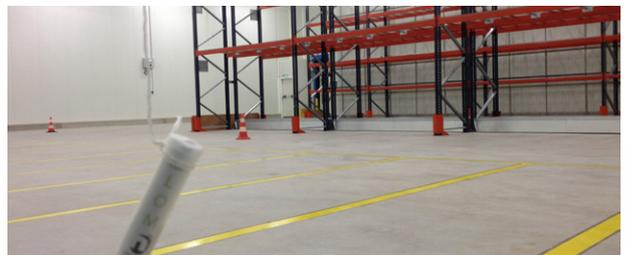
Installation in a warehouse for the realization of a thermal cartography. 75 temperature recorders deployed.
