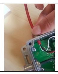
5. Connect the other vibrating wires following the same procedure and then close the enclosure.
