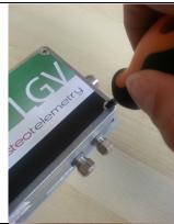
2. Unscrew the cable gland of the input you will connect
