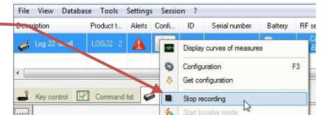
Wait a radio transmission or use the magnet on the logger so that the modification is taken in account by the logger. (The number of measurements in memory is displayed in the column "measures" of the line of Logger).
