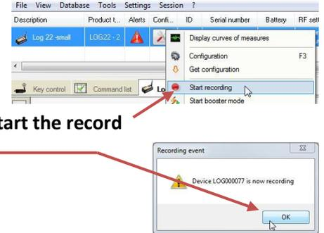
Wait a radio transmission or use the magnet on the logger so that the Logger takes changes in account. The measurement campaign begins; now the logger records all its measures in its memory and sends a signal every minute to indicate its presence and its state, exceedances of alert and the number of measurements in memory. **Make sure you get your measurements on the curve of measures** (at the period chosen for the recording mode).
