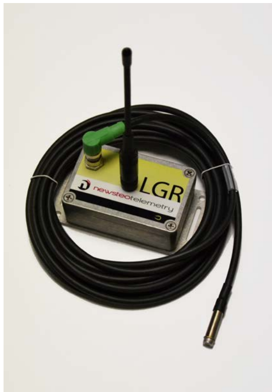
Figure 1: Example of a LGR data logger connected with an external probe
