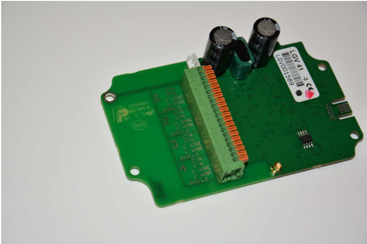
Figure 2: Vibrating wires connection
