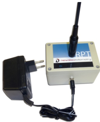
Figure 8: PFPN-RPT20-001- Repeater with main current power supply
